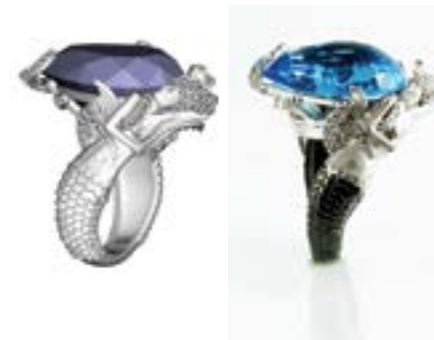
Mermaid Ring rendered in CAD and produced by CAMMING at ARCH by the students of Jewellery Design
